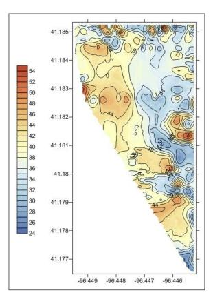
GSSI Profiler EMP-400 16 kHz conductivity plot showing variations in soil texture & moisture holding capacity at a known test plot. Data was collected with the system towed behind an ATV – note GPS positioning. Scale to the left shows the values represented in mS/m.
