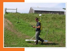
Picture shows complementary GPR system, UtilityScan™
