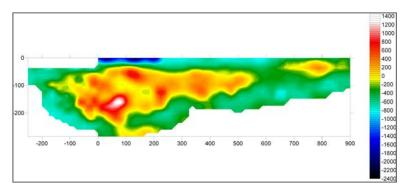
Soil conductivity map of a former landfill site indicating lateral extent of areas of high conductivity caused by landfill refuse.
