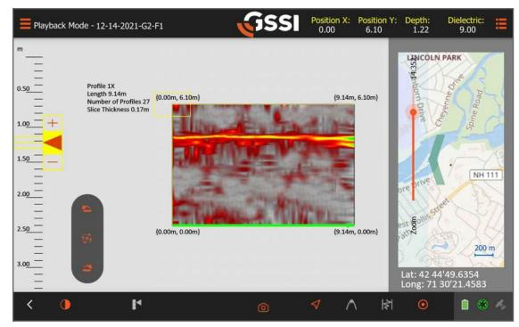
Data image shows a horizontal yellow line that is a water line located at 1.25m in depth, collected with 3D mode.
