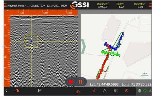
Data on the left side of the screen shows a typical utility at 1.25m in depth and shows a nicely defined base layer at .4m in depth. The blue dot on the data image is a water line.
